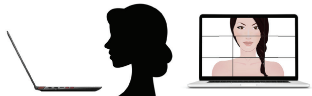
Example B - Screen tilted outwards ( incorrect )
